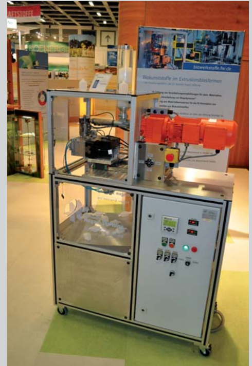
Initial small blow mould plant (constructed 2010) at the IGW Berlin in 2015
